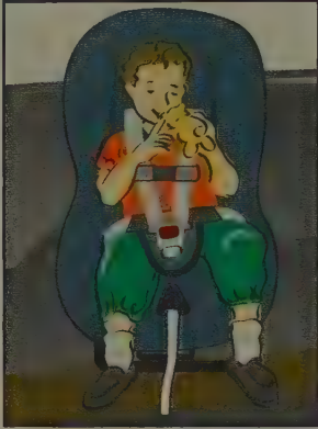
C. Children who are at least two and have outgrown their rear-facing seat can ride forward-facing.
