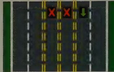
C Reversible lane at different times of day may be used by traffic moving in opposite directions
