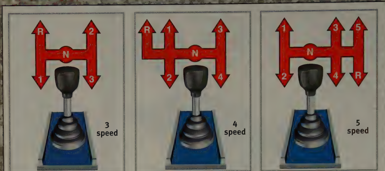
Cars with a manual transmission have a gearshift instead of a selector lever. The gearshift can have 3, 4, or 5 speeds.
